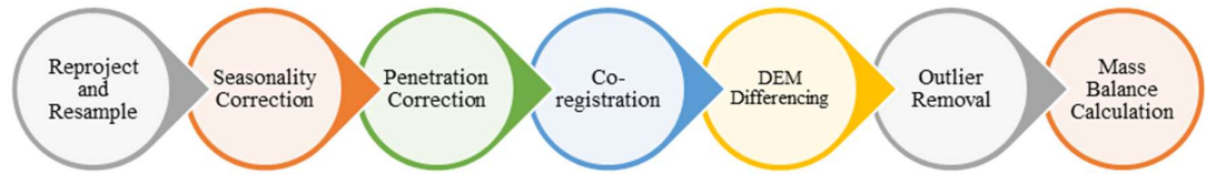
Fig. 4.2 Methodology for Geodetic Mass Balance Calculation
